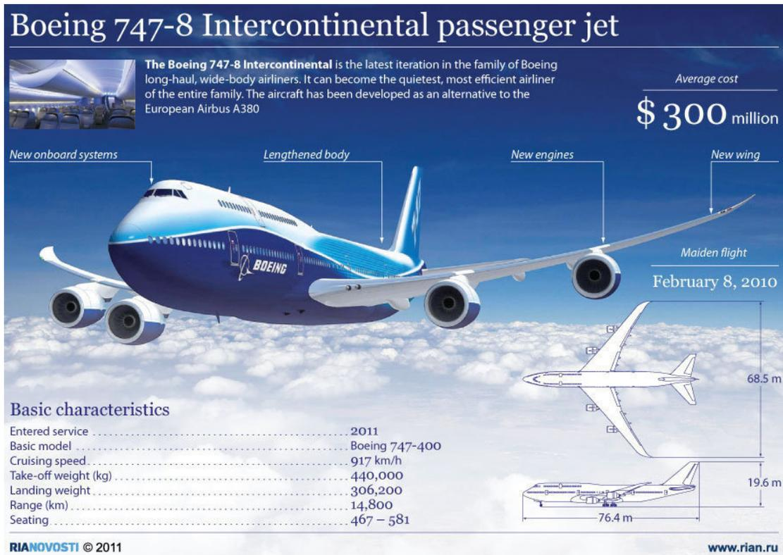
Figure 2. Boeing 747-8i design and key technical specifications
